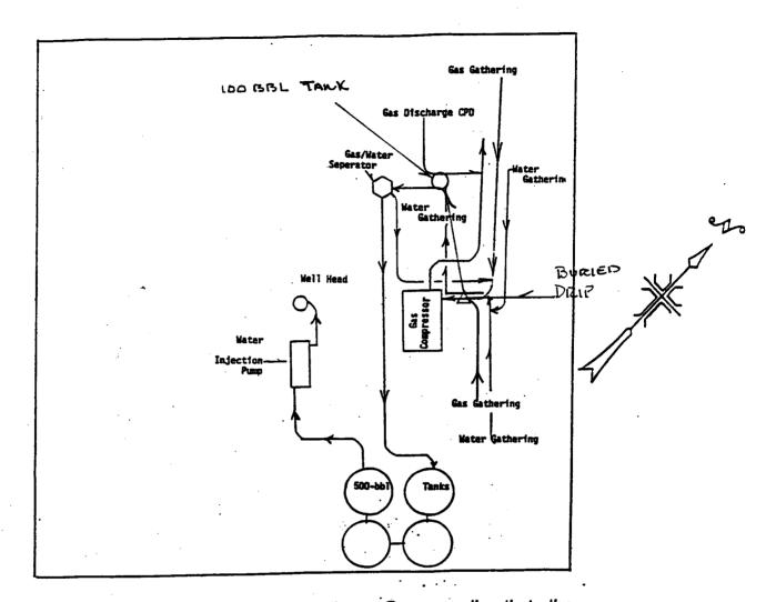
Gas and water come to location in separate lines. Gas goes directly to the compressor and the water goes through the separator. Separated water goes to the water storage and then to the injection pump. Water is then pumped into the disposal well. All gas is compressed and discharged to a C.P.D. on an existing El Paso gas gathering system.
