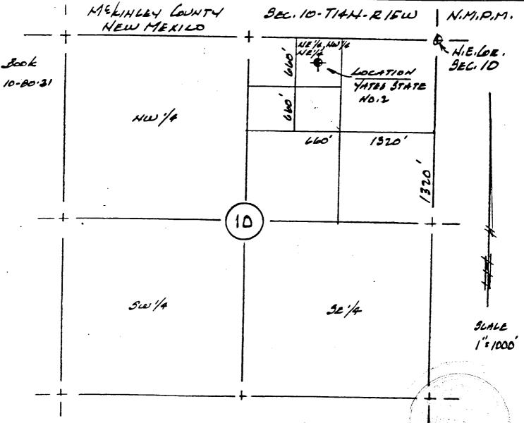
YATES STATE No. 2 IS LOCATED 1,588 PEEF WEST AND 318 FEEF SOUTH OF THE N.E. LOR. BEC. 10 - TIAM. RIEW NIM. P.M., IN THE NE'/4, NW /4, NR'/4 OF SEC. 10.
