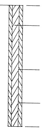
Plugged by filling with cement from bottom to top
