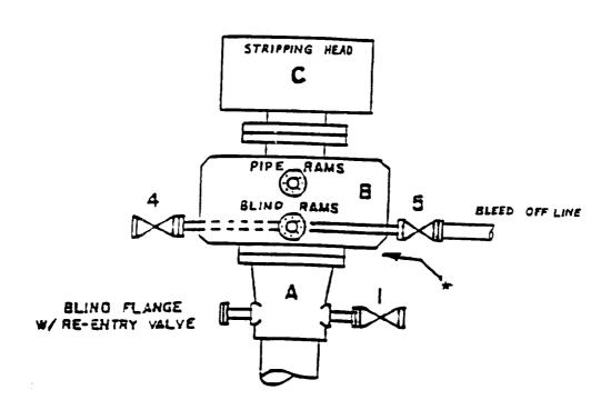
\*Where substructure height is adequate, a spool as per the specifications under Condition II will be added at this point and the kill and choke lines will be connected to the spool rather than rams.
