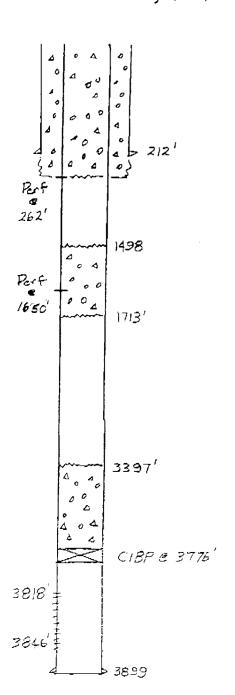
All cmt - Class B 15.6 \*/gal Speceffuld-water 11-5-01 MERU APIUS Well Service. TOH w/ tbg. Pickup 5/2" CIBP on tbg., set @ 3776! Load csg., presstest csg to 500 PSI for 10 min. Held. Spot 44 sx (51.9 fts) from 3397' to 3776!. TOH.
