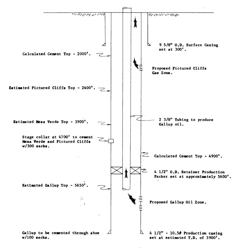
Note: Gallup oil zone to be produced through 2 3/8" tubing string. Pictured Cliffs gas to be produced up casing-tubing annulus.
