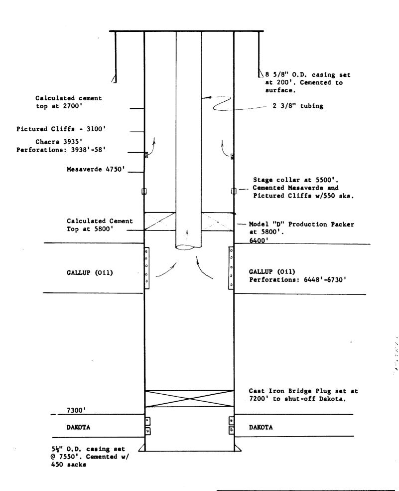
DUAL COMPLETION SCHEMATIC JICARILLA APACHE 30 WELL NO. 4 UNIT F, SECTION 31, T25N, R5W RIO ARRIBA COUNTY, NEW MEXICO
