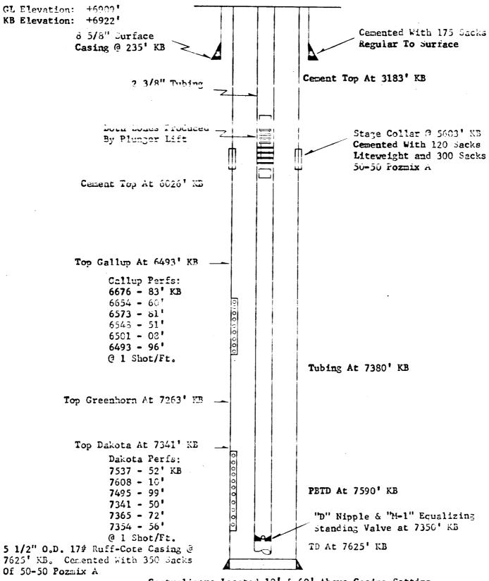
Centralizers Located 10' & 60' Above Casing Setting Depth and Every 90' Thereafter to 6475' KB; Also One Centralizer 30' Above and 30' Below Stage Collar.
