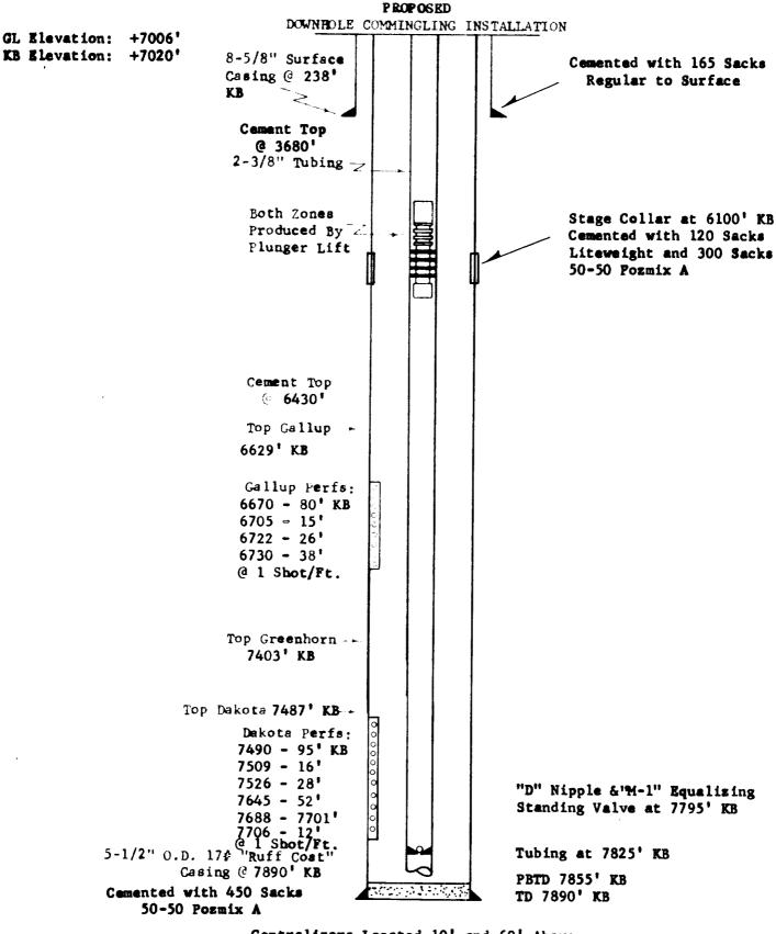
Centralisers Located 10' and 60' Above Casing Setting Depth and 90' Thereafter
