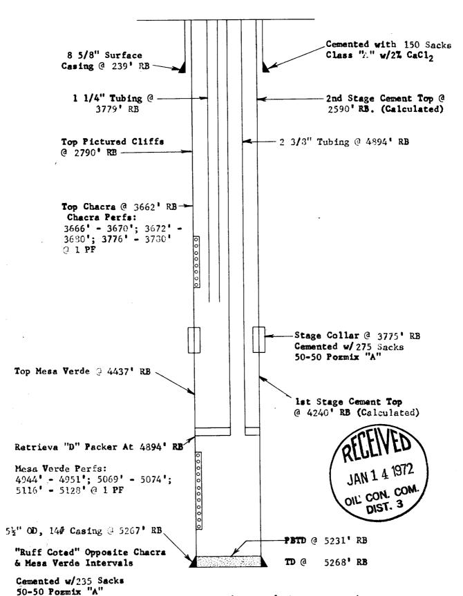
Centralizers at 10° and 60° above shoe and at 90° intervals to 2860° RB.
