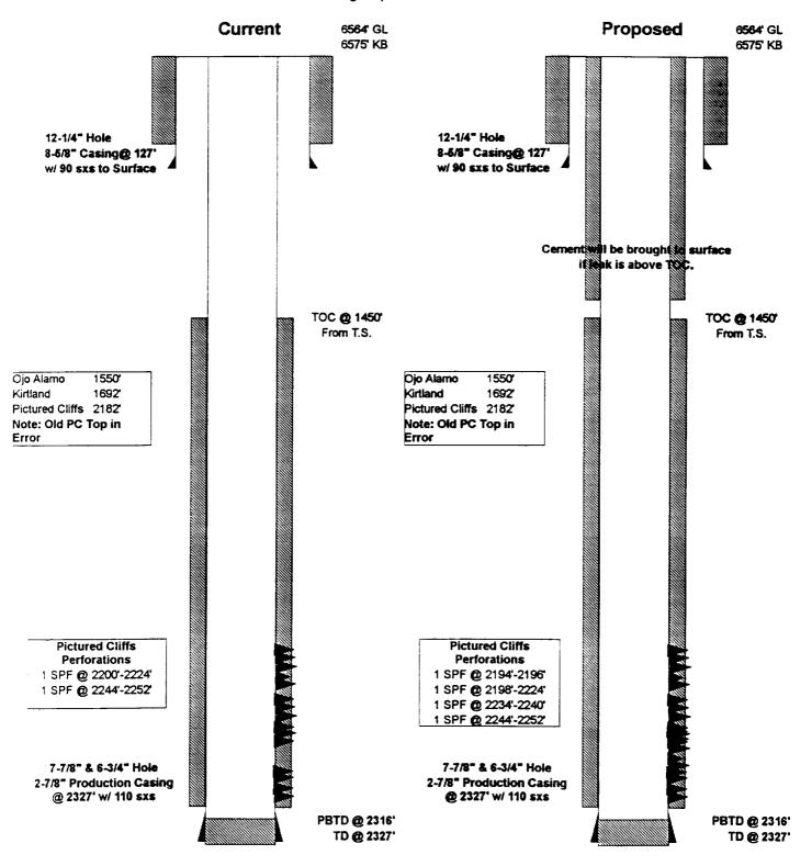
Well was perforated 1 SPF and fraced w/ 25,000# 10/20 sand @ 27 BPM. Well has a casing failure. This failure is most likely above TOC.
