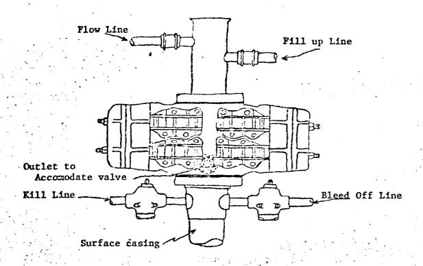
Blowout preventer is Shaffer double hydraulic equipped with drill pipe rams in the top and blind rams in the bottom.
