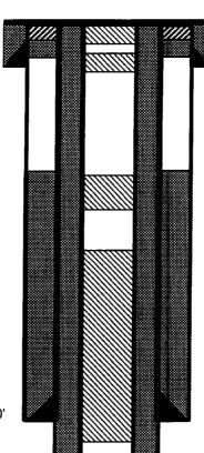
4-1/2" TOC at Surface, circulated 5 sxs cement; 8-5/8" TOC Unknown, 50 sxs(127') pumped into BH annulus, then took 8 bbls water to load (96' down)
