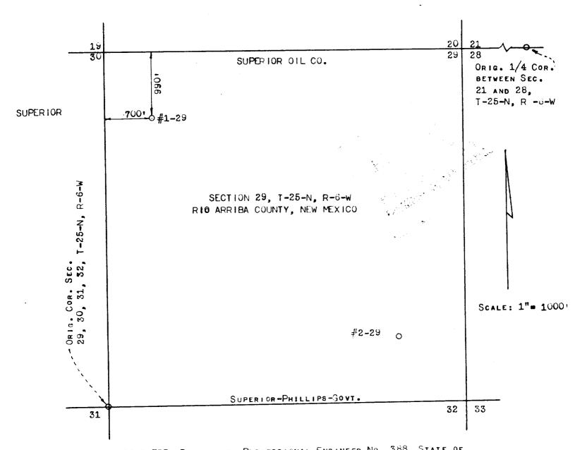
I, W W STUDDERT, REGISTERED PROFESSIONAL ENGINEER No. 388, STATE OF NEW MEXICO, HEREBY CERTIFY THAT THIS WELL LOCATION: SUPERIOR OIL CO., SUPERIOR-PHILLIPS-30VT., #1-29, 990' FROM THE NORTH LINE AND 700' FROM THE WEST LINE OF SECTION 29, T-25-N, R-6-W, RIO ARRIBA COUNTY, NEW MEXICO STAKED ON THE GROUND UNDER MY SUPERVISION AND THAT THIS PLAT IS DECEMBER 15, 1955
