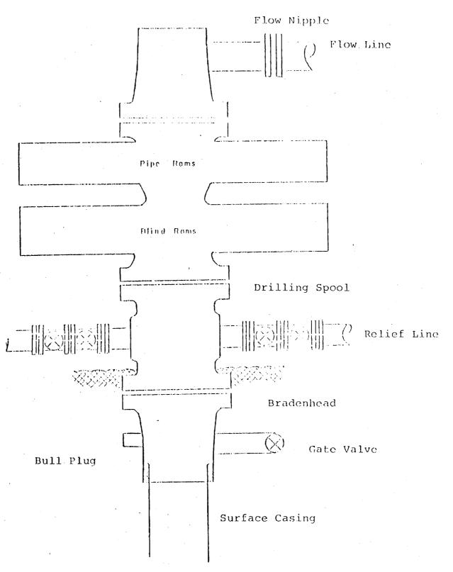
800 Series 900 Double Gate BOP, rated at 3000 psi Working Pressure
