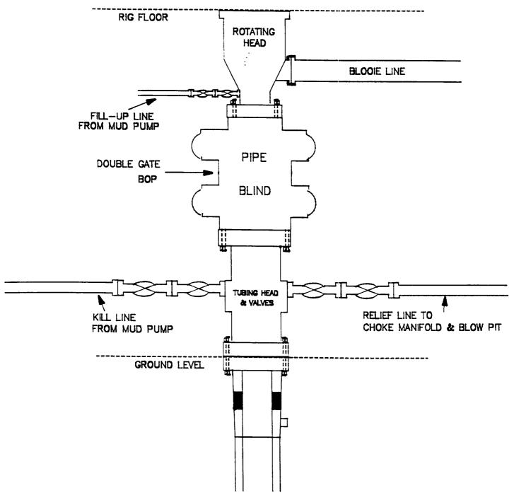
Minimum BOP installation for Completion operations.  $7 \frac{1}{16}$ " Bore (6" Nominal), 3000psi minimum working pressure double gate BOP to be equipped with blind and pipe rams.
