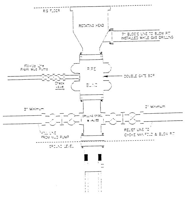
Minimum BCP installation for a Mesaverde well from Surface to Total Depth. 11" Bare, 2000psi minimum working pressure double gate BOP to be equipped with blind and pipe rams. A Schaffer Type 50 or equivalent rotating head to be installed on the top of the BOP. All equipment is 2000psi working pressure or greater.
