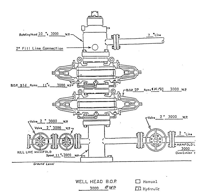
NOTE: Although 3000 psi BOP equipment will be used, equipment determination and line sizing are based on the requirements for 2000 psi BOP equipment due to the known drilling and reservoir conditions.
