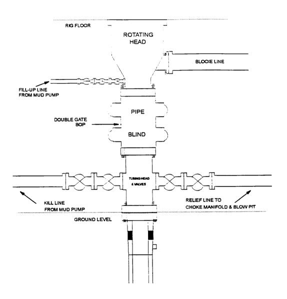
Minimum BOP installation for Completion operations. 7 1/16" Bore (6" Nominal), 3000 psi minimum working pressure double gate BOP to be equipped with blind and pipe rams.
