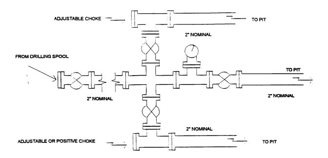
Minimum choke manifold installation from surface to Total Depth. 2" minimum, 2000psi working pressure equipment with two chokes.
