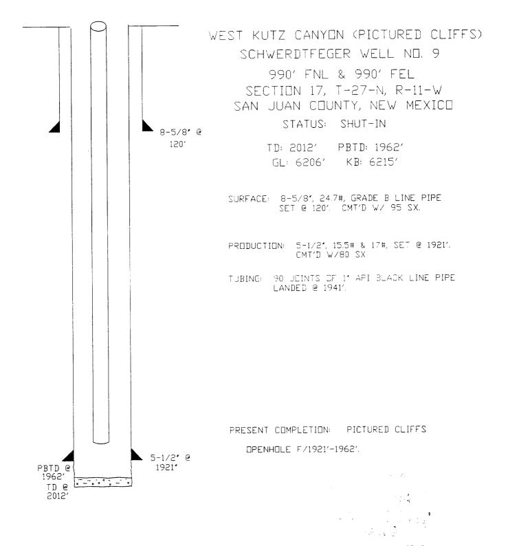
HISTORY: DRILLED IN JANUARY, 1952 BY FRONTIER REFINING COMPANY. COMPLETED IN PICTURED CLIFFS OPENHOLE F/1921'-1962'. TREATED W/50 QUARTS JELLED NITRO & 62 QUARTS LIQUID NITRO. SHUT-IN APRIL, 1986 AFTER PRODUCING 101 MMCF FROM PICTURED CLIFFS.
