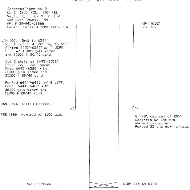
6444' - 6460' 4 SPF 6495' - 6502' Cut 3 Slots 6507' - 6512' Cut 3 Slots 6516' - 6520' Cut 3 Slots 6550' - 6565' 4 SPF
