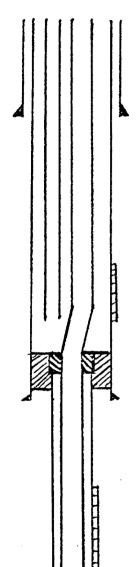
9-5/8", 36# casing set at 308'. cemented with 160 sxs.
