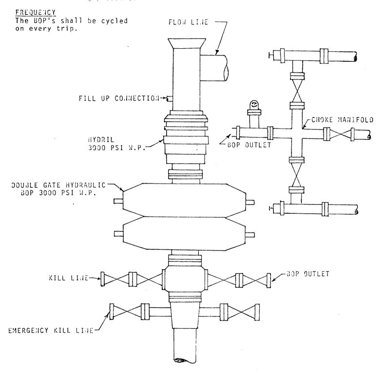
SCHEMATIC DRAWING 3000 PSI - BOP Equipment
