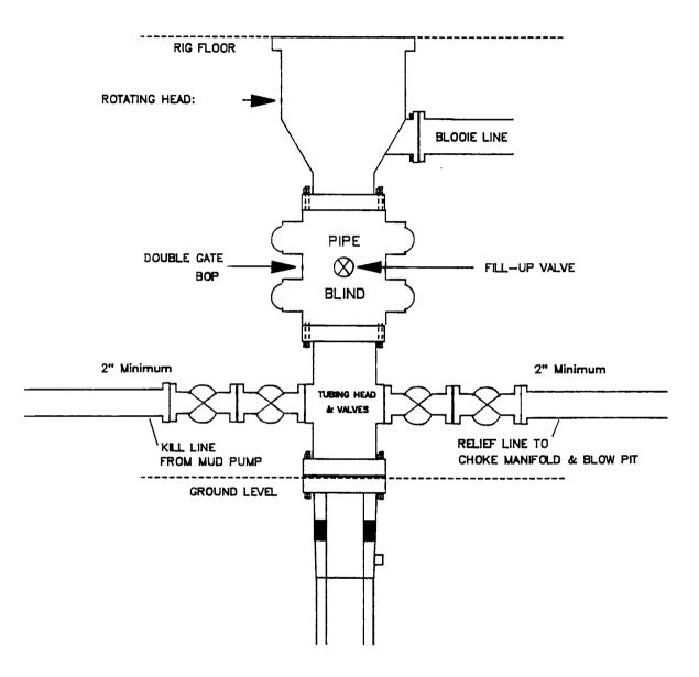
Minimum BOP installation for Completion Operations. 7 1/16" Bore (6" Nominal), 2000psi minimum working pressure double gate BOP to be equipped with blind and pipe rams.
