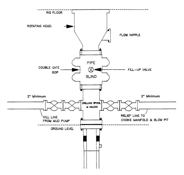
Minimum BOP installation for a typical Fruitland Coal well from surface to Total Depth. 11" Bore (10" Nominal), 2000psi minimum working pressure double gate BOP to be equipped with blind and pipe rams.
