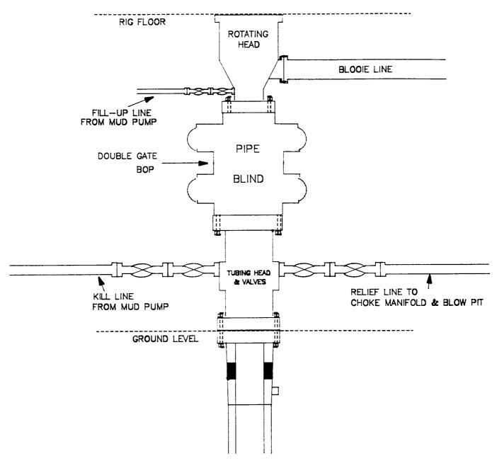
Minimum BOP installation for Completion operations.  $7 \frac{1}{16}$  Bore (6" Nominal), 3000psi minimum working pressure double gate BOP to be equipped with blind and pipe rams.
