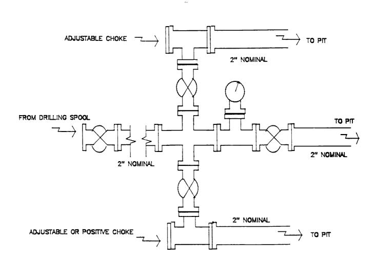
Minimum choke manifold installation from surface to Total Depth. 2" minimum, 2000psi working pressure equipment with two chokes.
