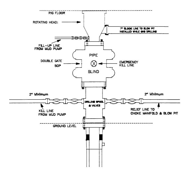
11" Bore, 2000psi minimum working pressure double gate BOP to be equipped with blind and pipe rams. A Schaffer Type 50 or equivalent rotating head to be installed on the top of the BOP. All equipment is 2000psi working pressure/or greater.
