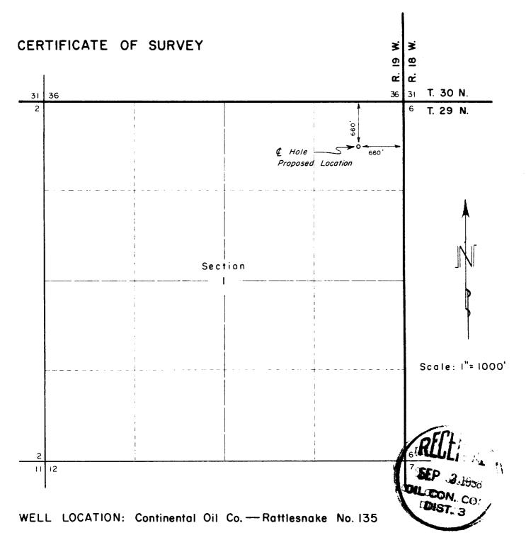
Located 660 feet South of the North line and 660 feet West of the East line of Section I.
