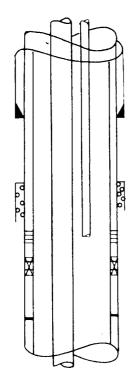
I" EUE KOBE TUBING HUNG @ ± 3300 FOR MESAVERDE UNLOADING STRING 2 3/8 EUE TUBING SET @ ± 6220 FOR DAKOTA PRODUCTION
