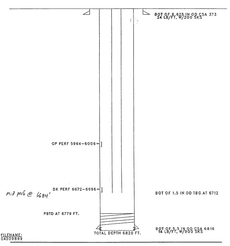
3/5/85 SQ 368-520 W/118CUFT CLASS B CEMENT 3/5/85 SQ CASING LEAK @494 W/90CUFT
