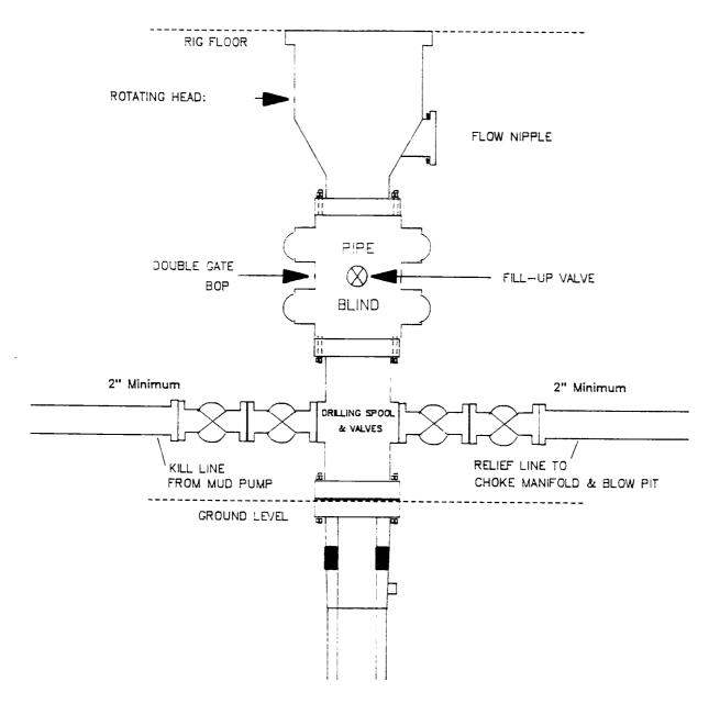
Minimum BOP installation for a typical Fruitland Coal well from surface to Intermediate casing point. 11" Bore (10" Nominal), 2000psi minimum working pressure double gate BOP to be equipped with blind and pipe rams. A Schaffer Type 50 equivalent rotating head to be installed on the top of BOP. All equipment is 2000psi working pressure/or greater.
