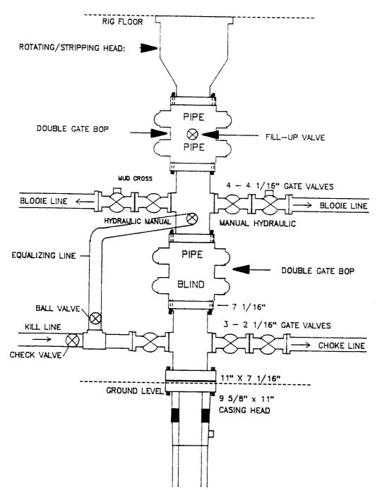
Minimum BOP installation for a typical open—hole Fruitland Coal well from intermediate TD to TD. 7 1/16" Bore (6" Nominal), 2000psi working pressure/ or greater double stack double gate BOP equipped with three pipe and one blind ram.
