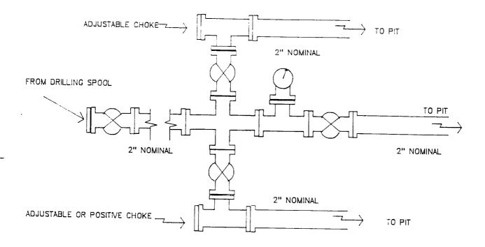
Minimum choke manifold installation for a typical Fruitland Coal well from surface to Total Depth. 2", 2000psi working pressure equipment with two chokes.
