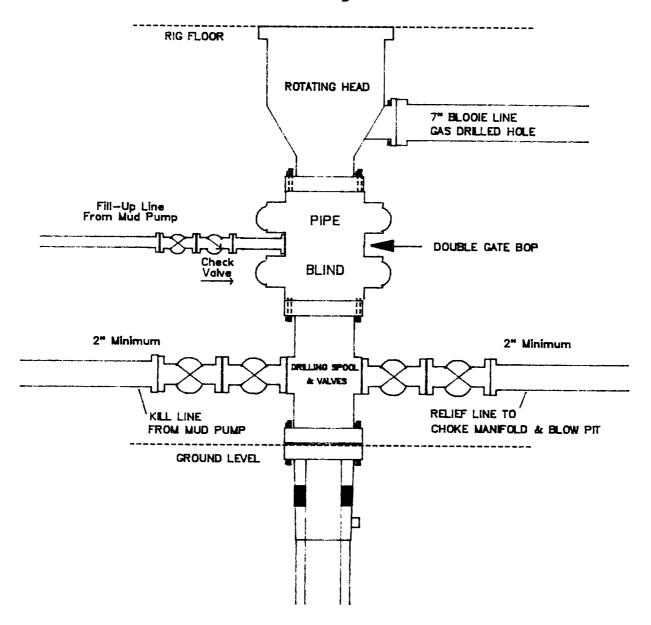
Minimum BOP installation for the Riddle #1R Mesaverde well from Surface to Total Depth. 13 3/8" Bore, 2000psi minimum double gate BOP to be equipped with blind and pipe rams. A Schaffer Type 50 or equivalent rotating head to be installed on the top of BOP. All equipment is 2000psi working pressure/or greater.
