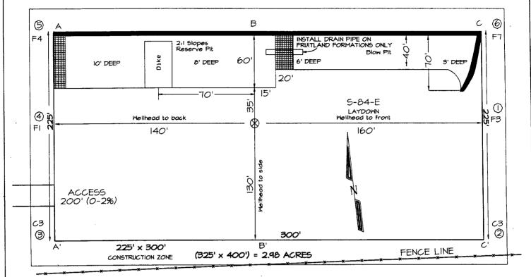
Reserve Pit Dike: to be 8' above Deep side (overflow ~ 3' wide and 1' above shallow side). Blow Pit: overflow pipe halfway between top and bottom and to extend over plastic liner and into blow pit.
