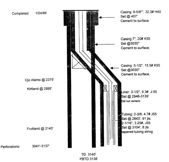
Workover History: 4/93 Install PCP 5/97 Remove rods & PCP rotor 6/97 RU for recav.,
