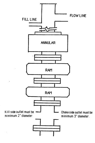
Kill line will be minimum 2" diameter and have 2 valves, one of which shall be a minimum 2" check valve.
