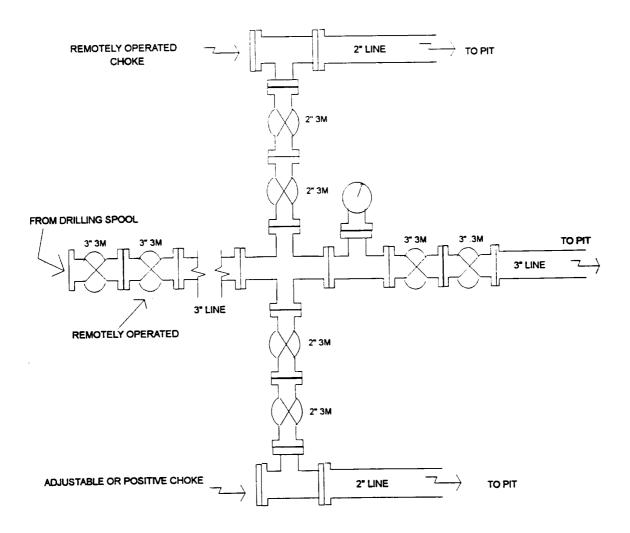
Choke manifold installation from surface Casing Point to Total Depth. 3,000psi working pressure equipment with two chokes.
