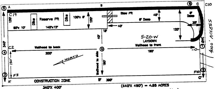
Reserve Pft Dike : to be 8' above Deep side: ( overflow - 3' wide and 1' above shallow side. ) Blow Pit : overflow pipe halfway between top and bottom and extend over plastic ilner and into blow pit.
