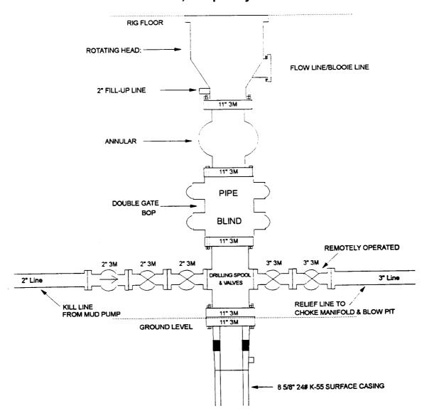
BOP installation from Surface Casing Point to Total Depth. 11" Bore (10" Nominal), 3,000psi working pressure double gate BOP to be equipped with blind and pipe rams. A 3,000psi Annular preventer to be installed on top of rams. A rotating head on the top of Annular preventer. All BOP equipment is 3,000psi working pressure.
