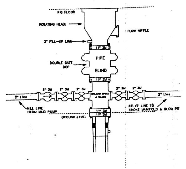
11" Bare (10" Nominal), 3000psi working pressure minimum double gate BOP to be equipped with blind and pipe rams. A rotating head on the top of the rams. All BOP equipment is 3000psi working pressure.
