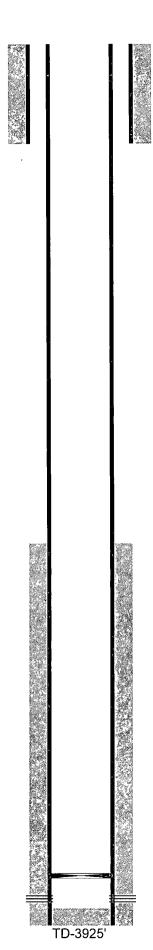
12-1/4" hole @ 437' 8-5/8" csg @ 437' w/ 325sx-TOC-Surf-Circ
