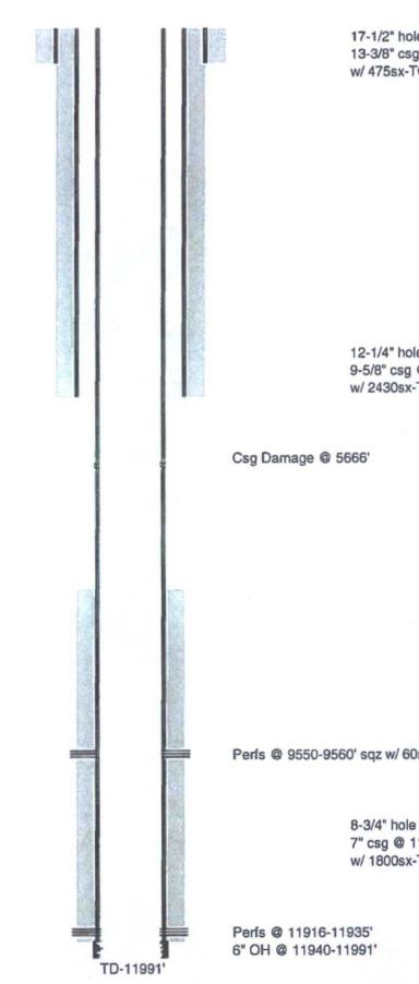
17-1/2" hole @ 449' 13-3/8" csg @ 449' w/ 475sx-TOC-Surf-Circ
