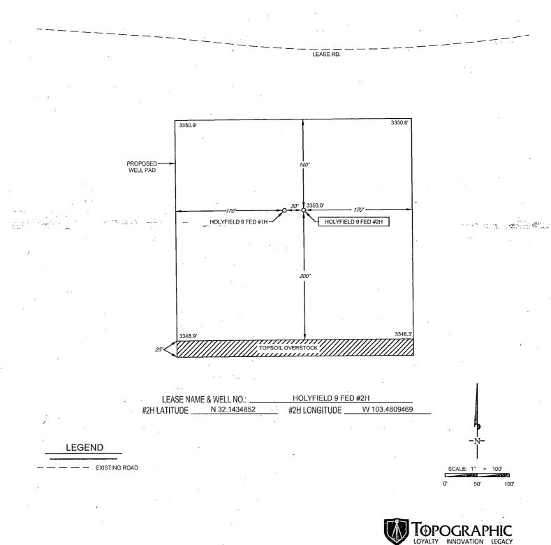
ALL BEARINGS, DISTANCES, AND COORDINATE VALUES CONTAINED HEREON ARE GRID BASED UPON THE NEW MEXICO STATE PLANE COORDINATE SYSTEM, EAST ZONE OF THE NORTH AMERICAN DATUM 1927, U.S. SURVEY FEET
