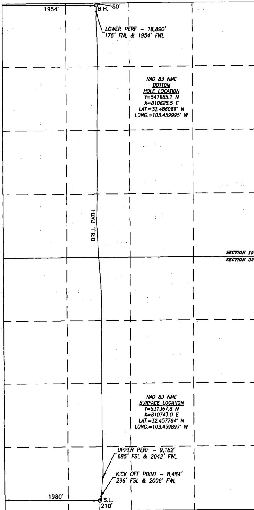
BOREPATH SHOWN HEREON IS BASED ON DIRECTIONAL SURVEY REPORT PROVIDED BY COG OPERATING, LLC FOR THE LYCHEE STATE COM #3H SUPPLIED TO HARCROW SURVEYING, LLC ON APRIL 15, 2019
