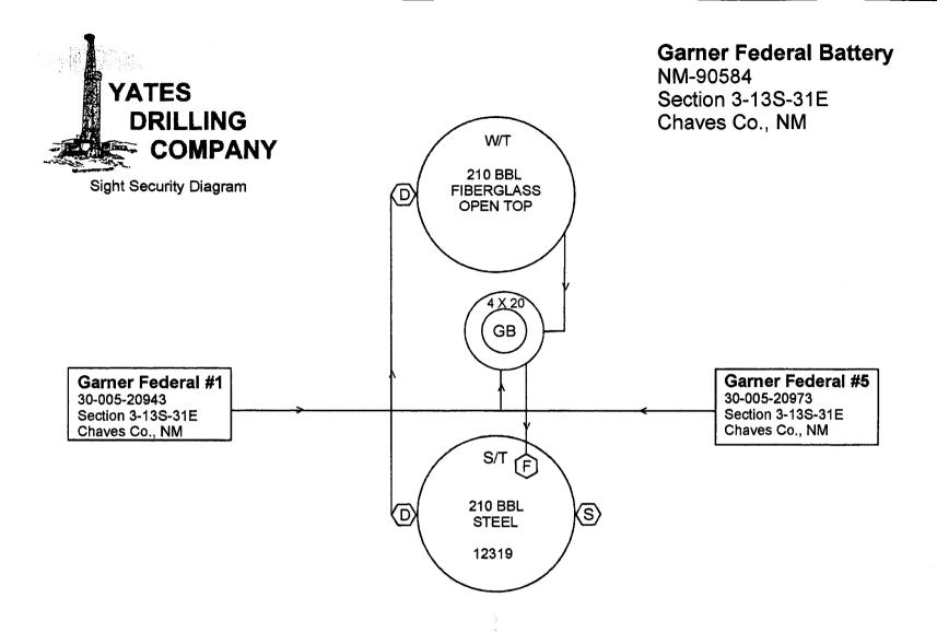
Production phase. All drain valves and all sales valves sealed closed.
