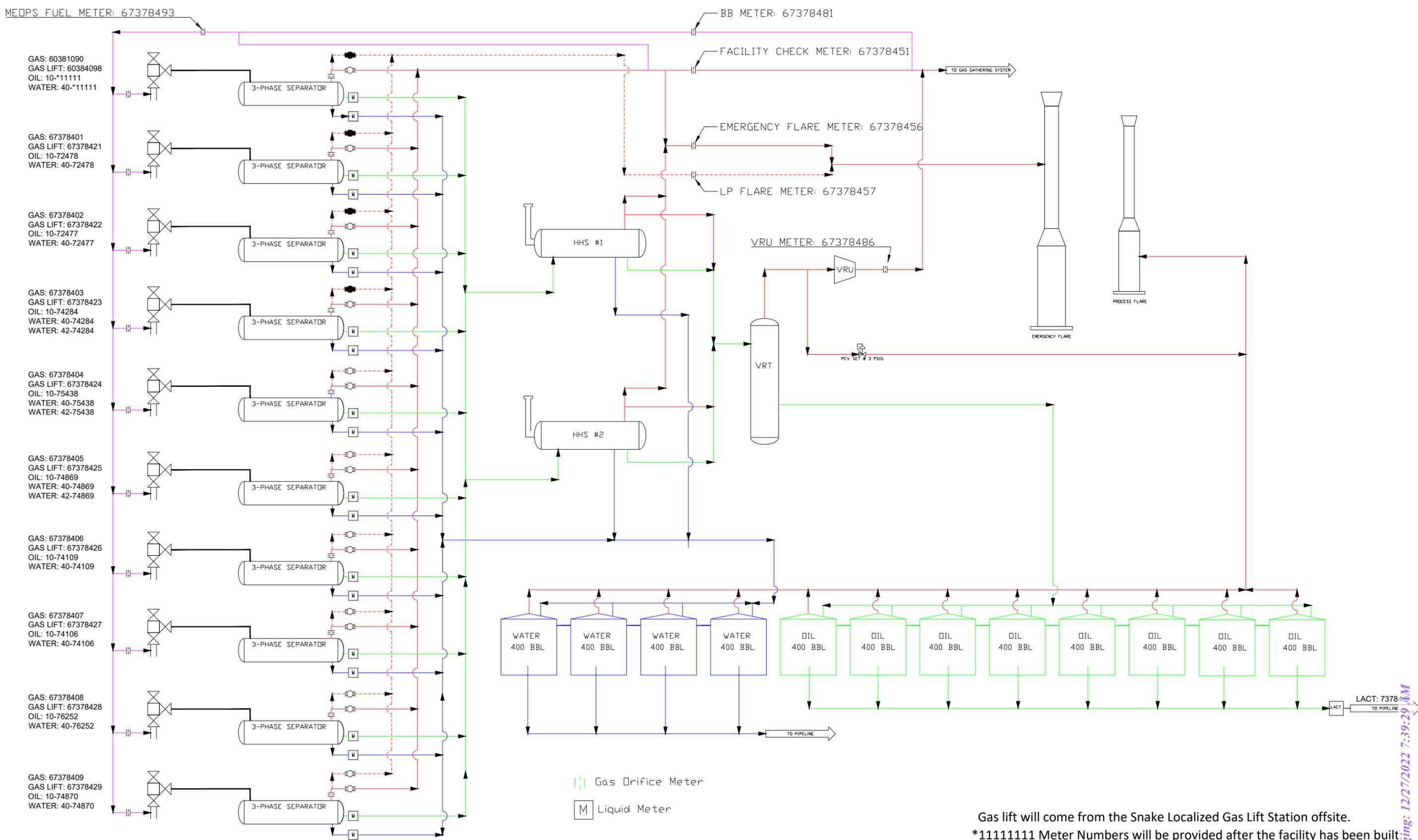
Gas lift will come from the Snake Localized Gas Lift Station offsite.
