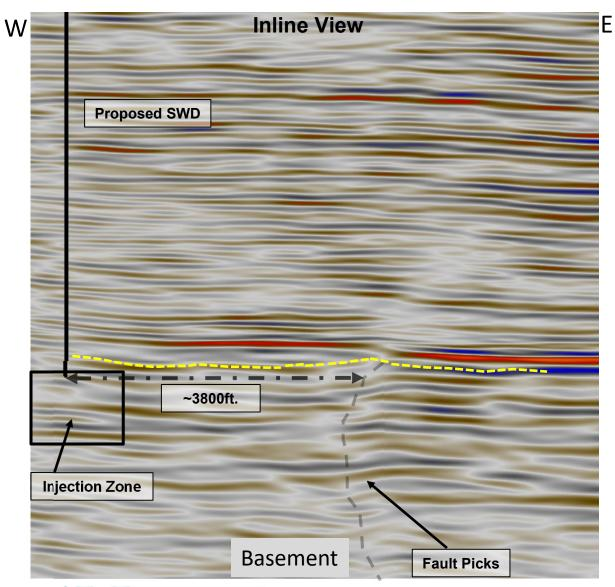
Near vertical faults observed on seismic on inline (E-W) view at ~3800 ft. east of proposed Rita SWD #1.
