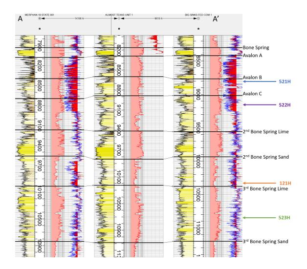
**Exhibit B-2** Cross-section A to A'. Stratigraphic cross-section hung on top of Wolfcamp. Target interval indicated by well number.
