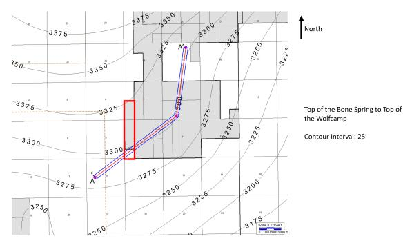
**Exhibit B-3** is a gross thickness map from the top of Bone Spring to the top of the Wolfcamp with a 25' contour interval. Map demonstrates a general thickness increase in the Bone Spring increasing to the northwest and decreasing the southeast as it pertains to the map extents.
