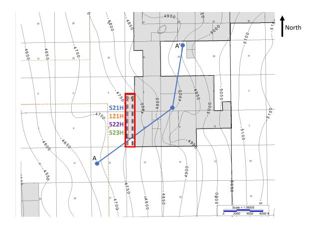
**Exhibit B-1** is a structure map showing the depth (subsea) of the top of the Bone Spring, a marker that is representative of overall structure for the development.
