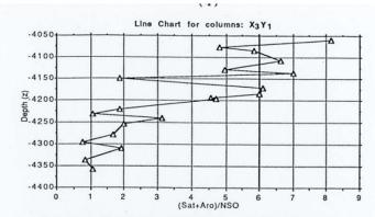
The sum of the saturates and aromatics can be related to the more mobile components of oil. Using the % NSO compounds as the denominator,(immobile component) a ratio of mobile (vs) immobile is calculated and plotted by depth. Again the same breaks in the depth curve occur as shown in the previous plots.
