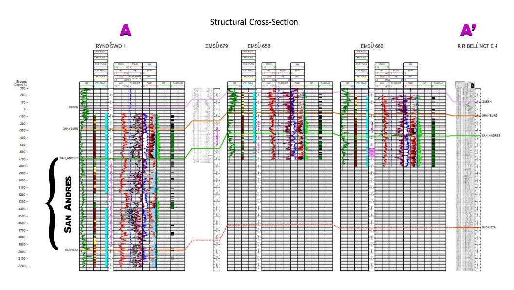
Log sections are based on NuTech's original analysis
