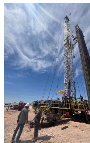
Figure 3. Modern Plugging Rig
