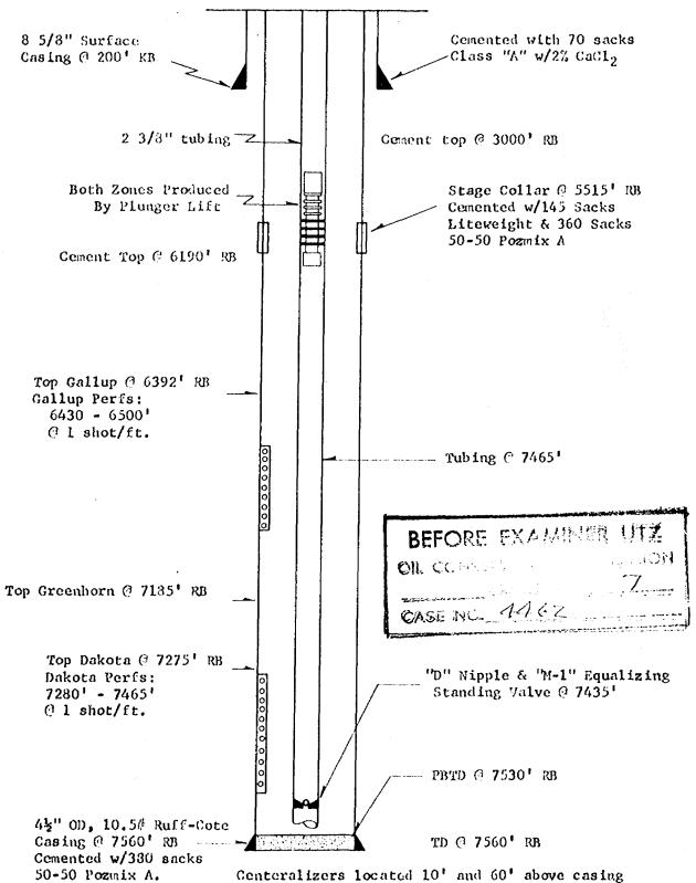
Centeralizers located 10' and 60' above casing setting depth and 90' thereafter to 6600' RB. Also, one centralizer 30' above and 30' below stage collar.
