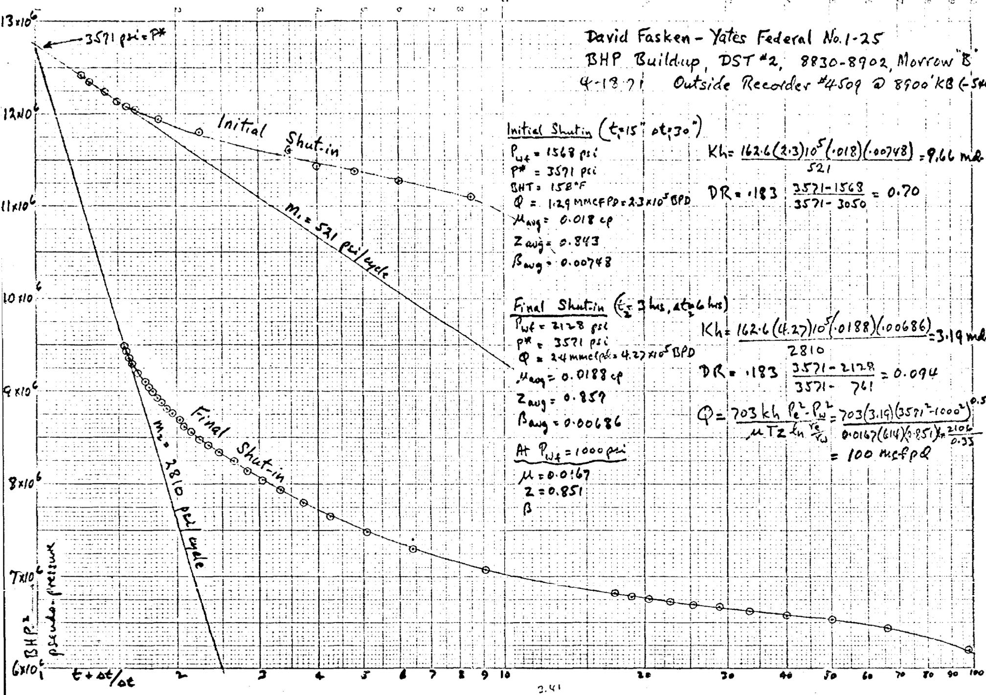
Initial Shut-in ( $t_1 = 15''$  at  $t_2 = 30''$ )
