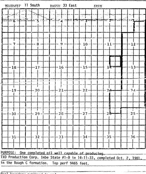
TXO Production Corp. Inbe State #1-B in 14-11-33, completed Oct. 2, 1981, in the Bough C formation. Top perf 9465 feet.
