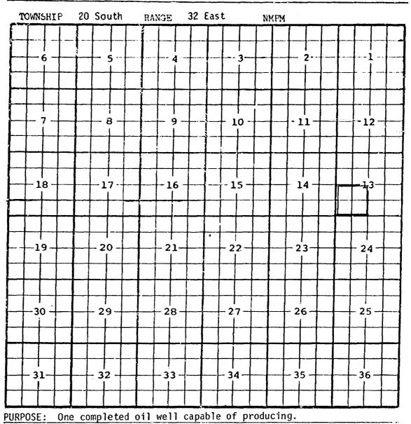
DISCOVERY WELL: Flag-Redfern Oil Company Hanson State #1-N, Sec.13-T20S-R32E. Completed in the Bone Springs formation on January 31, 1976. Top of the perforations 10,267'.
